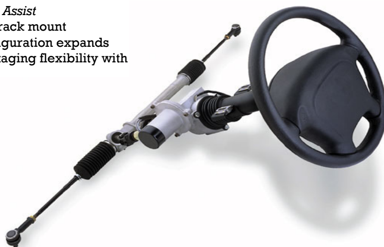
E-Steer system (Source: Delphi)
