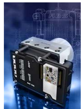
A modern hydraulic modulator and control electronics
